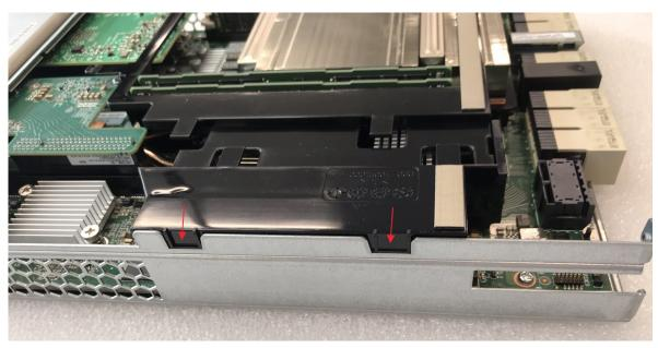
7. Put and close the case cover according to the below picture and put back in the two screws.
