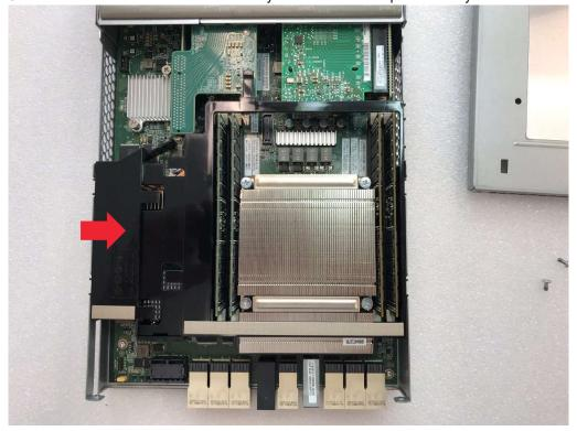
4. The M2 Disk including the PCI-carrier board can be removed without any tools or unlocking.
