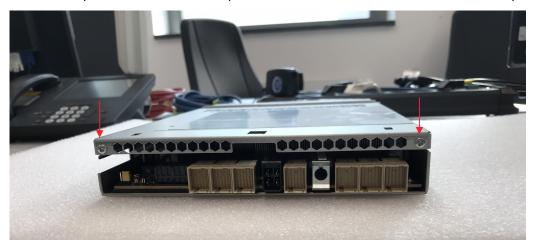
3. The black air-flow deflector can be easily removed vertical up without any tools.
