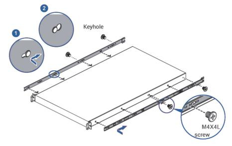
5. Continue installing the outer rail bracket to the mounting frame. Attach the outer rail assembly to the frame and press the bracket to fix the rail onto the frame.
