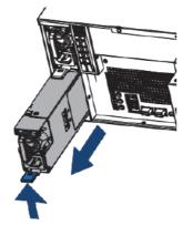
4. Slide the new unit into the power supply until it clicks into place.
