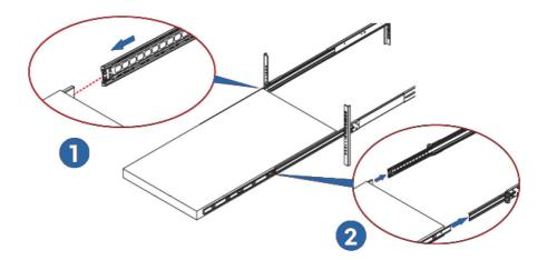
7. CAUTION! Verify the ball bearing retainer is locked.
