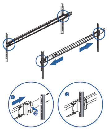
6. Pull out the middle channel until the ball bearing retainer is locked forward.
