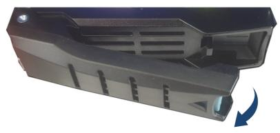
**4.** Pull the tray lever outward completely and remove the disk carrier out of the system.
