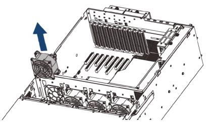
2. Insert the replacement fan into the node. Make sure to align the rubber connectors with the appropriate slot in the bracket.
