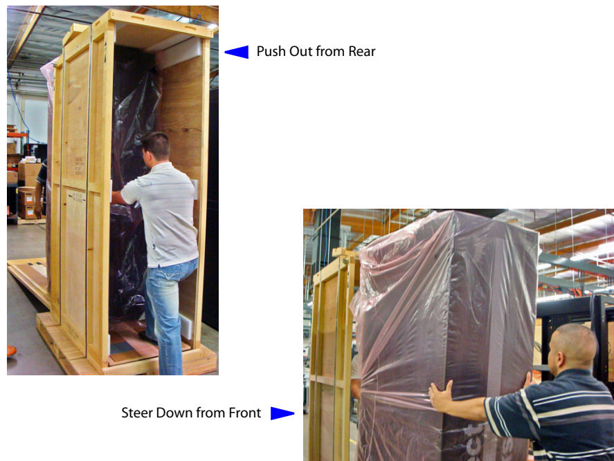
Figure 14. Pushing Out the Rack
