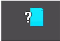
Spycer shows all files available on the storage, even files of unknown formats. Files that are not recognized by Spycer are displayed with this icon (text information as well as thumbnail view). However, because each will be worth one entry in the database of the SpycerAgent, your storage should contain as few of these files as possible. Otherwise search procedures may get lengthy due to unnecessary overhead.
