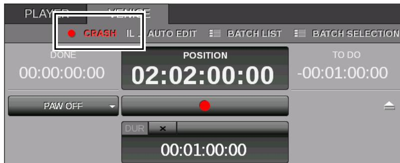
Figure 4-19: The operating elements in the crash record mode
