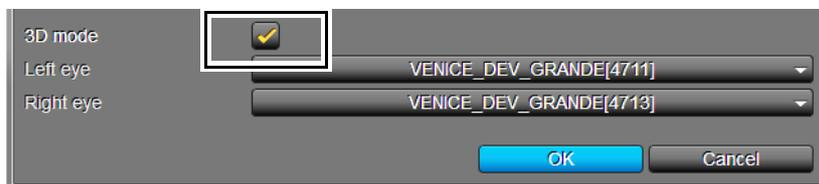
Figure 4-7: Setting the 3D mode
