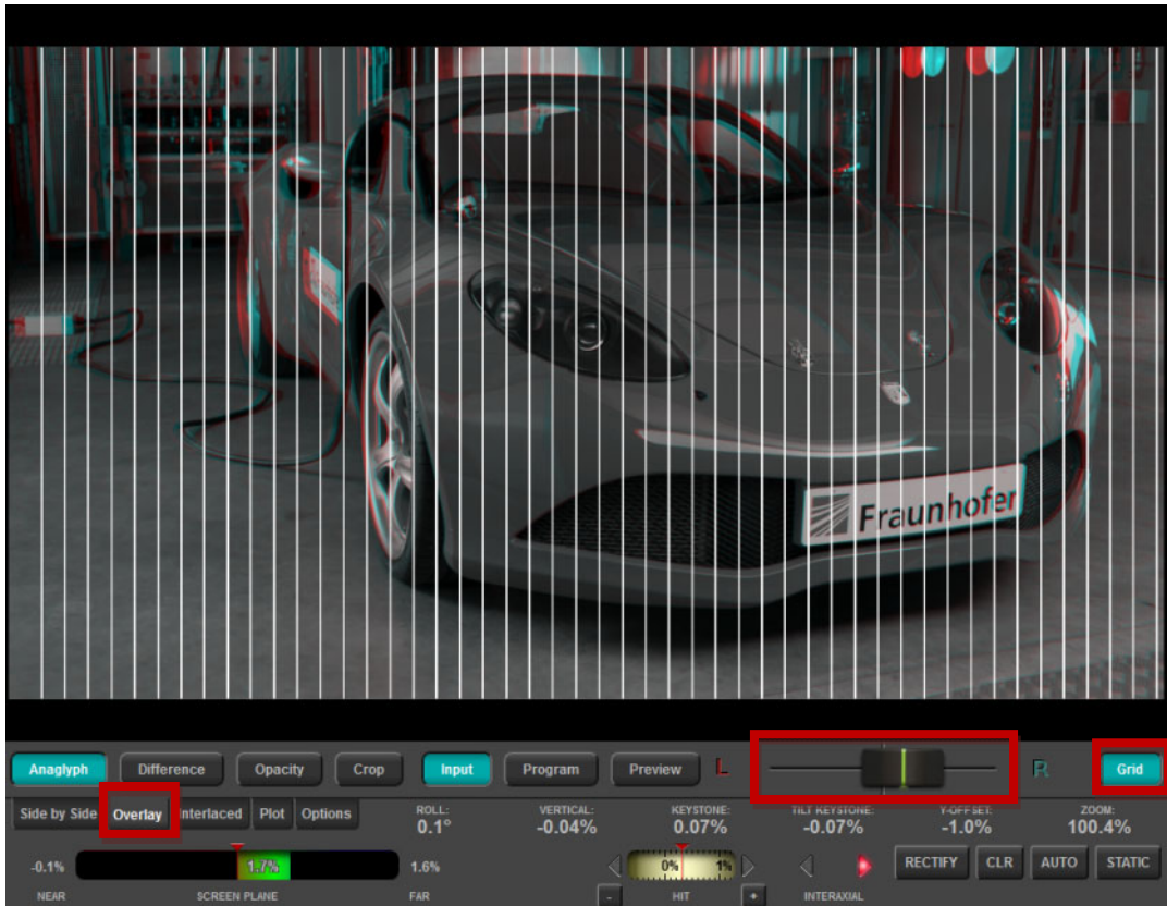
Figure 4-2: Grid lines applied to an Anaglyph Overlay image. Each grid line corresponds to a disparity of 2% of the image width. Use the slider to move the grid lines left and right. The sensor shift (or HIT) can be used to bring the near clipping plane or the far clipping plane to convergence.
