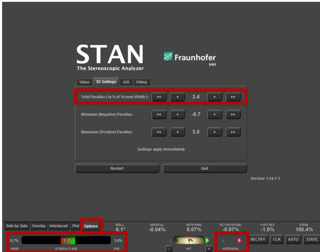
Figure 4-3: The Depth Volume (1.7% in this example) is compared to the Depth Budget (Total Parallax to be defined in the Options menu). Subsequently STAN derives in which direction the interaxial distance needs to be changed. In this example the red arrow to the right indicates that the interaxial distance needs to be increased drastically. If you increase the Depth Budget (i.e. Total Parallax), STAN will take this into consideration and suggest higher interaxial distances.
