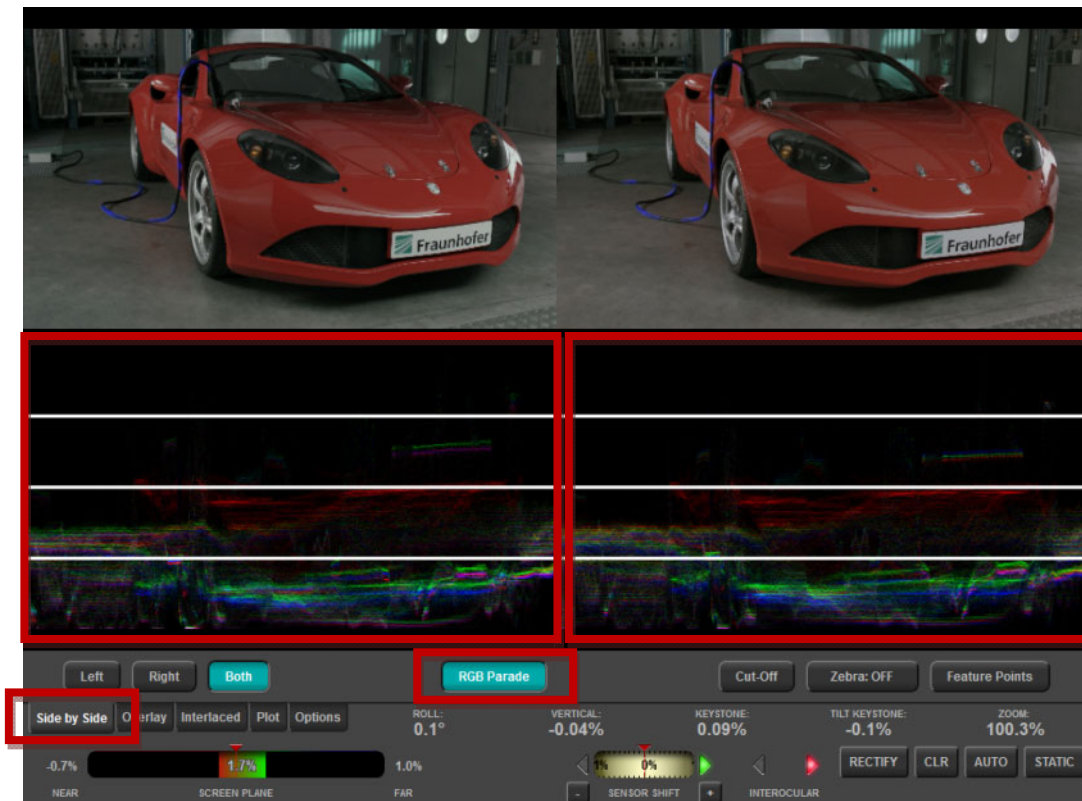
Figure 5-1: RGB Parade. This visualization option is useful to match the color temperatures and/or the iris settings of the two cameras.
