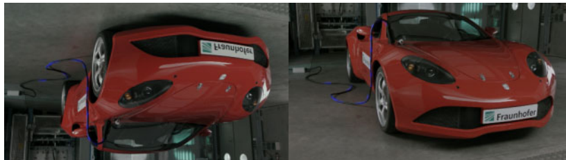
Figure 2-3: Unmodified camera signals. The left image is flipped due to the use of a mirror rig while shooting the content. Using the Side-by-Side view mode, one can easily see the flipping option that is required.
