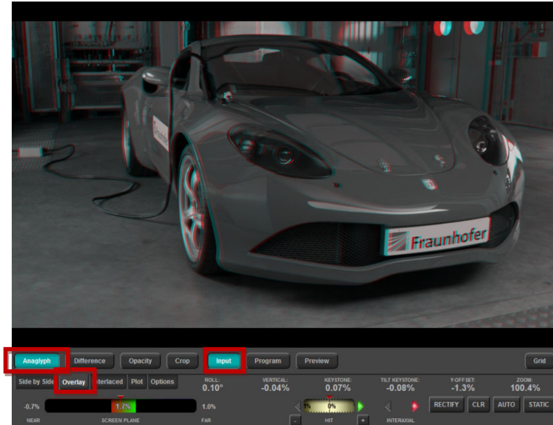
Figure 3-2: The Anaglyph Overlay mode can be used to get a visual feedback of the quality of the mechanical alignment. Red or cyan lines around horizontal object borders in the image are clear indicators for the presence of vertical disparities and thus for a poor mechanical alignment.
