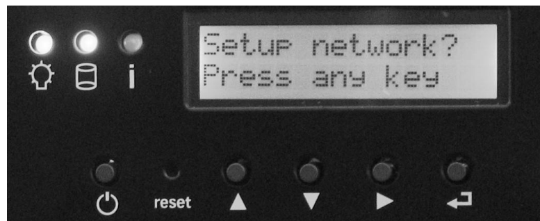
Figure 1. If LCD shows this message press any of the four control keys enter network setup.
