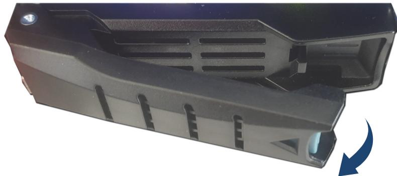
4. Pull the tray lever outward completely and remove the disk carrier out of the system.
