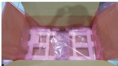
4. Place the system into the box with the front pointing to the right and wrap it completely with the ESD foil.
