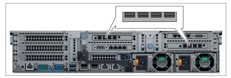
To use the functionality you have to insert the dual receiver and the dual transmitter into the SFP+ ports. For more information see chapter "Installing the System" on page 58.
