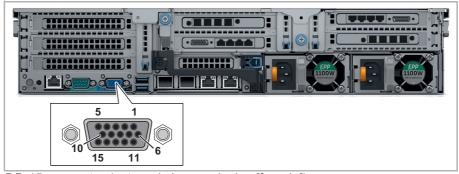
DB-15 connector (external view on device [female])
