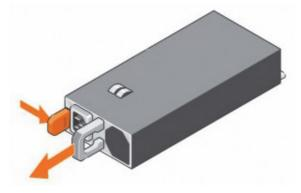
**3**. Slide the new PSU into the chassis until the PSU is fully seated and the release latch snaps into place.
