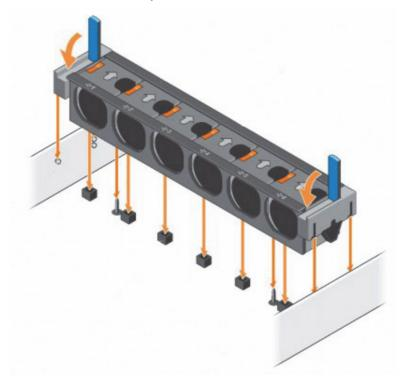
5. Lock the new cooling fan assembly into the chassis by lowering the release levers until firmly seated.
