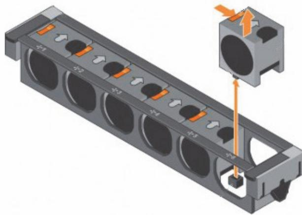
2. Align the connector at the base of the cooling fan with the connector on the system board.
