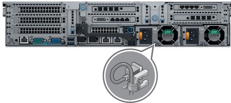
7. Connect a network cable to the Ethernet connector “eno3” or “eno4” depending on your installation routine. For details see chapter “Network Configuration” on page 63.
