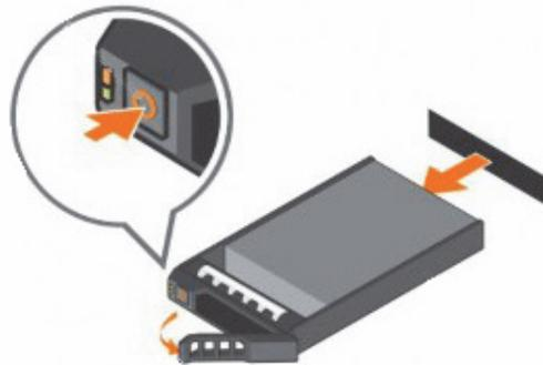
2. Slide the hard drive out of the hard drive slot.
