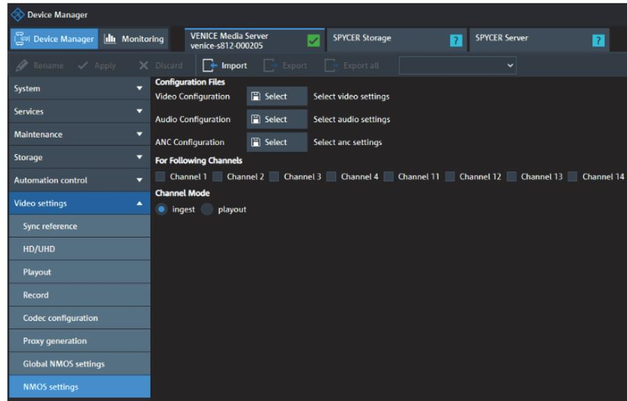
2. Import the JSON files with the NMOS configuration settings. There is one JSON file per data type, operation mode (playout or ingest), and channel.
