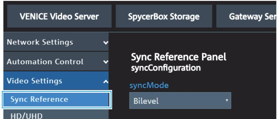
2. Set the **Sync Mode**, the **syncHPhase** and the **syncVPhase** as needed. For detailed information see the documentation of the R&S®Device Manager.
