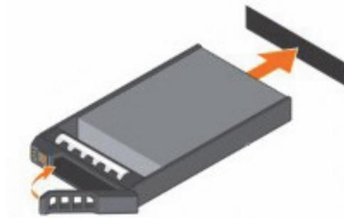
6. Close the hard drive carrier handle to lock the hard drive in place.
