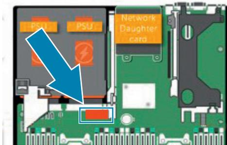
2. Insert the replacement USB memory key into the USB port.
