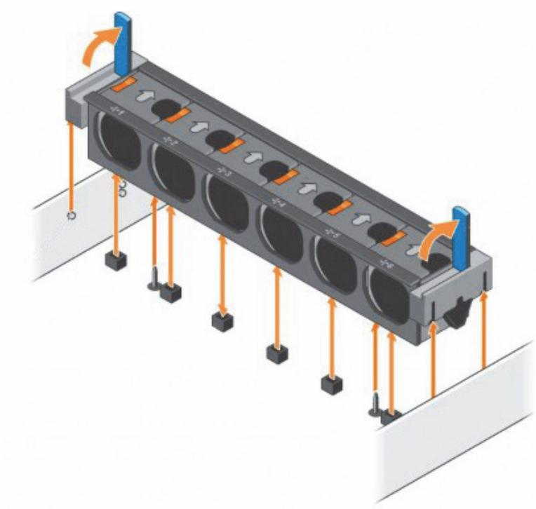
3. Align the slots on the cooling fan assembly with the guide pins on the chassis.
